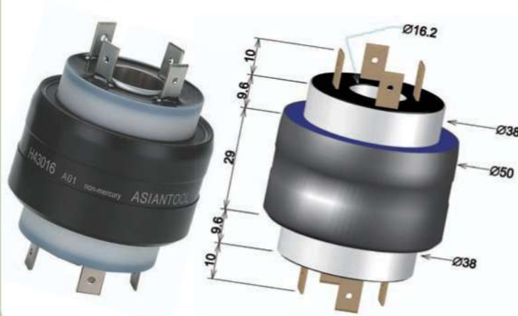
H43016 NM (non-mercury) 4poles/30A/AC250V Through-bore:16.2mm
