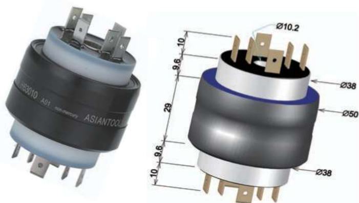
H63010 NM (non-mercury) 6poles/30A/AC250V Through-bore:10.2mm
