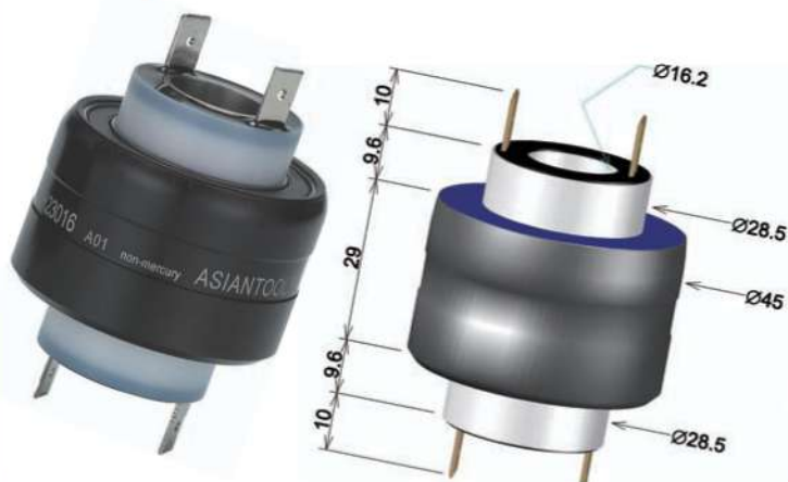
H23016 NM (non-mercury) 2poles/30A/AC250V Through-bore:16.2mm
